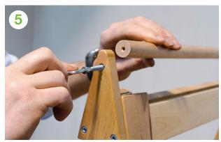
Assemble one end of the paper roll holder by tightening a woodscrew into the pre-drilled hole on the end of the paper roll holder.
