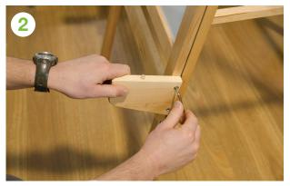
Assemble paint holder brackets with woodscrews into the pre-drilled holes on the side of the easel and repeat on remaining sides.
