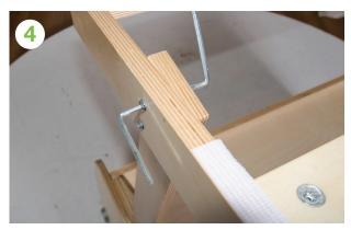
Tighten long bolts into insert nuts with 2x Allan keys provided. Repeat steps 1 and 2 on opposite end.
